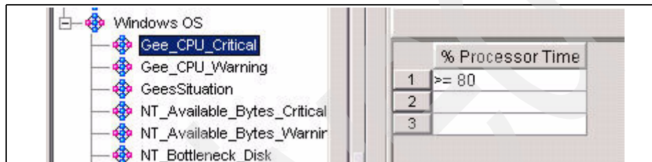
Figure 10-37 Situation that triggers when % Processor time \geq 80\%
